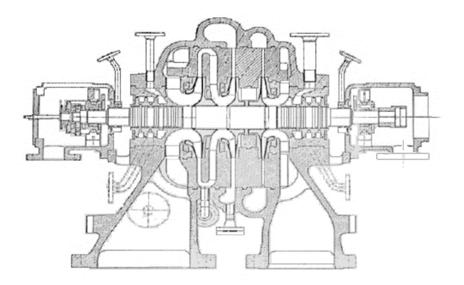
Figure 2 The cross-sectional view of the original compressor
