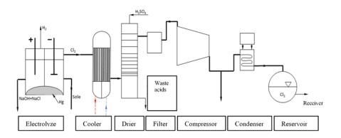
Figure 1 Simplified technological scheme of chlorine production by electrolyze of aqueous salt solution by Kramer [3]
