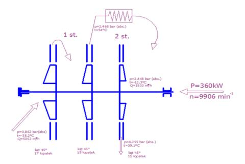
Figure 4 Calculation model of the chlorine compressor
