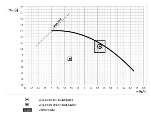
Figure 5 Results of modernized machine acceptance test
