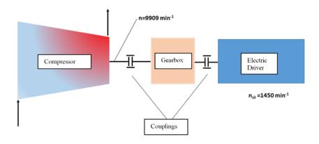
Figure 3 Compressor location with respect to the gearbox and electric motor
